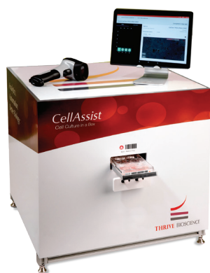
CellAssist Benchtop Imager Size 0.5m x 0.5m x 0.5m Weight 22kg
